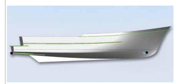
Despite the larger displacement, tank tests indicate that the design of the hull and the increased waterline length will deliver fuel consumption similar to the Fleming 55.
