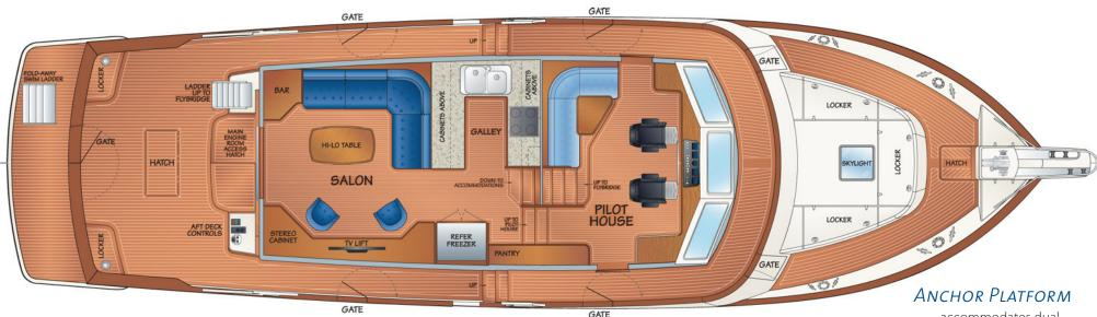
LARGE ACCESS HATCH into the engine room is just aft of the salon doors.
