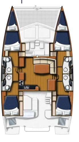
The Leopard 44 is available in either a 3 cabin, 3 head version, or a 4 cabin, 4 head version. Both layouts offer the option of additional storage, berth, or head in the forward hull.
